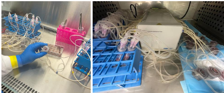
Figure 6-3. Assembly of bioreactor chambers and circuits in biological safety cabinet. Bone cores were put into the bioreactor chambers the day after bone core excision and preparation.
