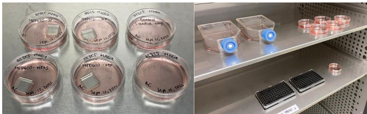
Figure 5-1. Rectangular constructs with the 4 different cleaning and sterilization protocols (MP, AP, SP, and SP+A) used for the sterilization screening protocol study.
