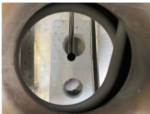
Figure 3.23: Radiometer positioning for cone calorimeter experiment.
