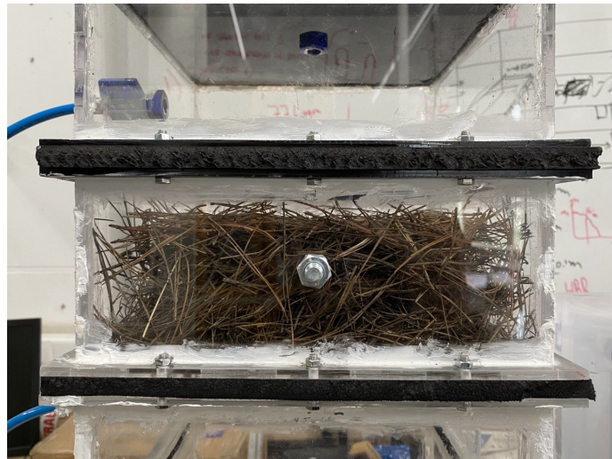
Figure 4.2: Example of fuel bed packing for pressure drop experiments to achieve permeability results.
