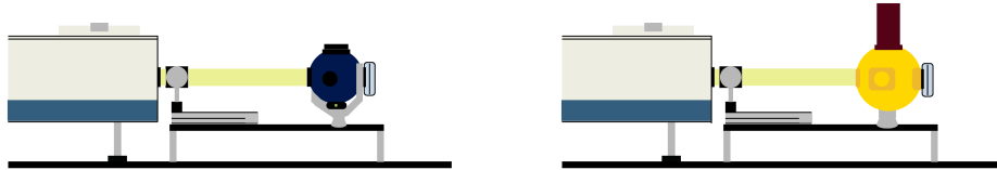
(a) Reflectivity setup, white sphere and biased detector.
